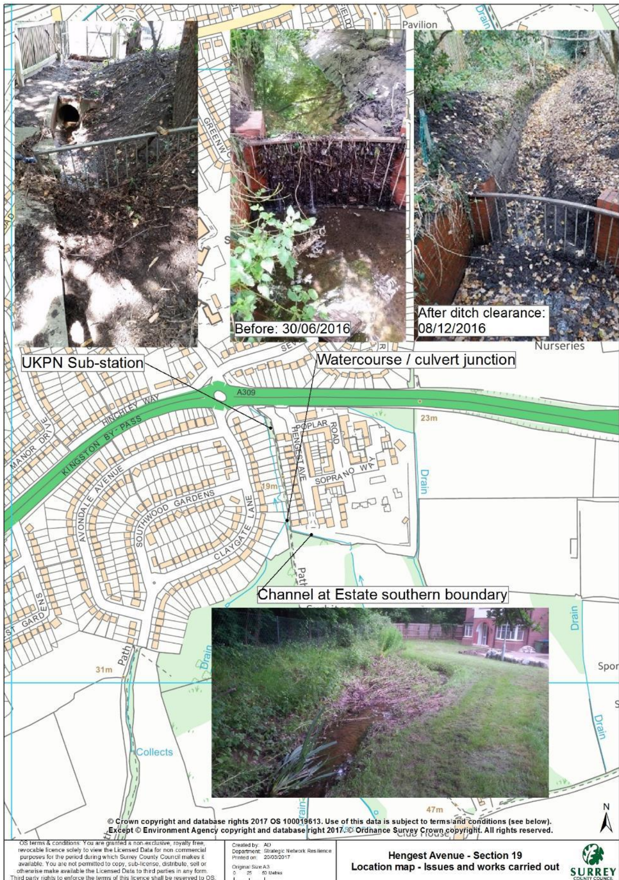
Figure 6. Location map summarising watercourse issues and works carried out. Photos taken as part of the SCC ME-252184 flood enquiry including before and after photos of the ditch clearance west of Hengest Avenue.
